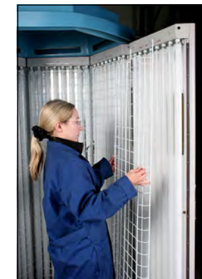
Unclip and remove screens.
